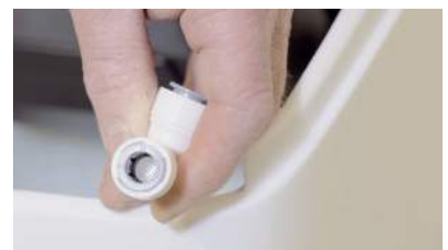
Replacement of brine discharge elbows
